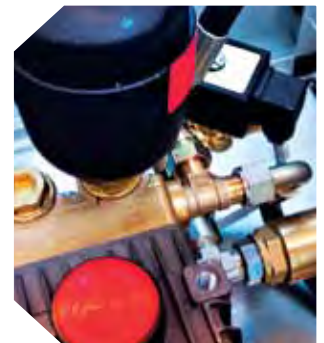
Detail of the high pressure pump of the Industriale 120 adjustable fog module.
