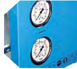
Detail of the pressure gauges to control air and water pressure.
